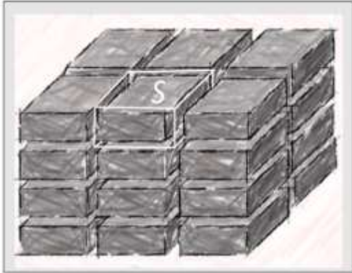
Figure 1: Schematic presentation of a planar conglomerate of HAPNs (shaded boxes) separated one from other by hydrated nanolayers. Supercell S is shown with white lines.
